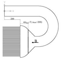
Fig.2. The perforated plate installed in the sodium channel inlet header
