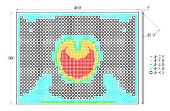
Fig. 6. The design of the perforated plate.
