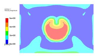
Fig. 5. Velocity contour at distance a=100mm (B view in Figure 2)
