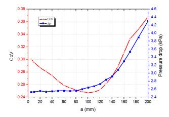
Fig. 4. The change of CoV and pressure according to distance a.
