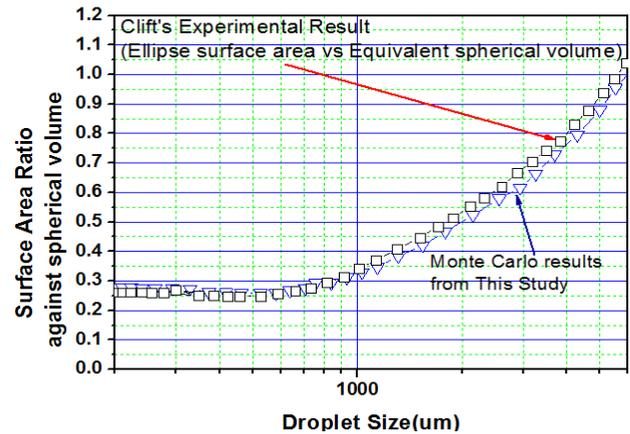
Fig. 2 Surface area ratio against spherical volume comparing with other study
