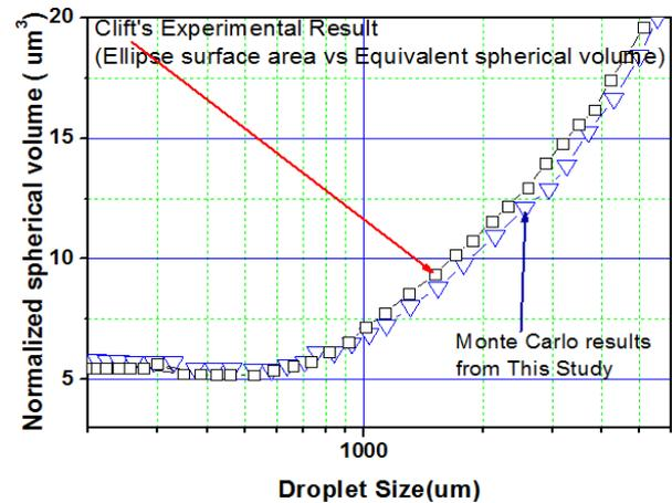
Fig. 3 Spherical volume and droplet size
