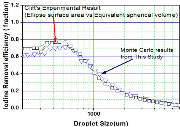
Fig. 5 Fission-products removal efficiency from ellipse surface area
