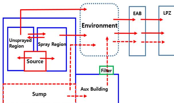
Fig. 1 LOCA modeling concept in RADTRAD code
