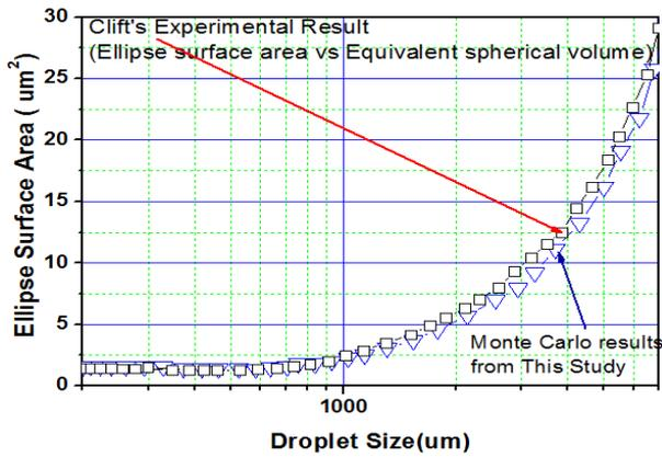
Fig. 4 Ellipse surface area and droplet size
