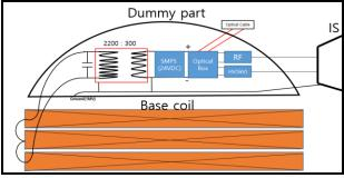
Figure.2 .Installation of the Ion source power system
