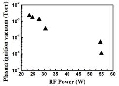
Figure. 5. Plasma ignition vacuum according to the RF input power
