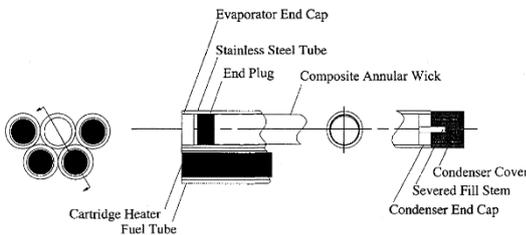
Fig. 2. Cutaway view of sodium heat pipe used for the LANL experiment [10].
