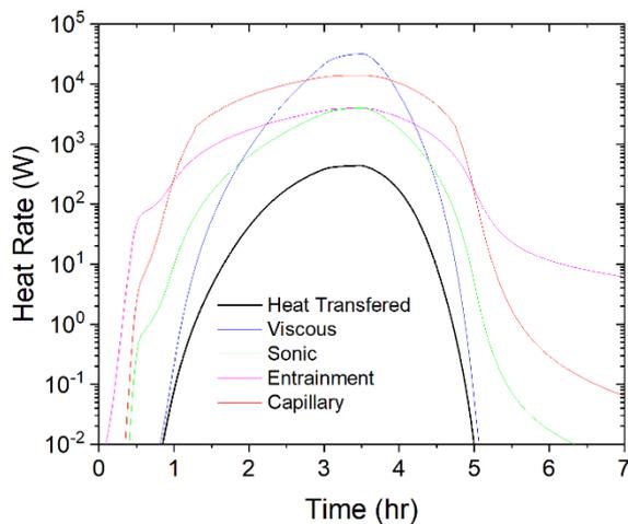
Fig. 5. Calculated vapor heat transport and operational limits of the heat pipe.
