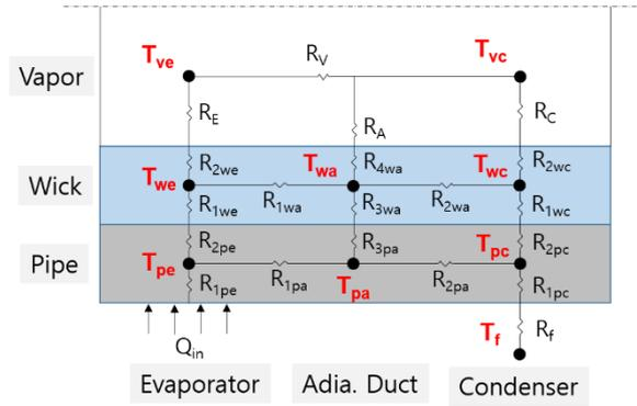
Fig. 1. Thermal network of the present heat pipe model.
