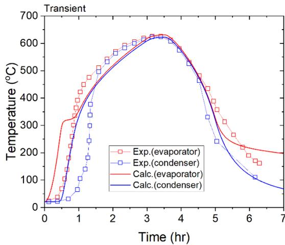
Fig. 4. Comparison of the predicted and measured surface temperatures of the heat pipe.
