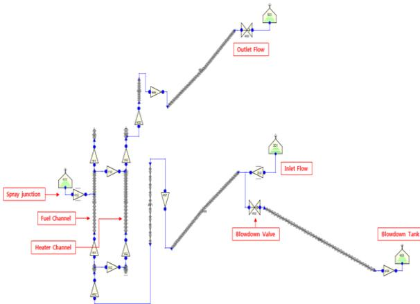
Fig. 2. Nodalization of test section for the assessment of IFA-650.9 experiment
