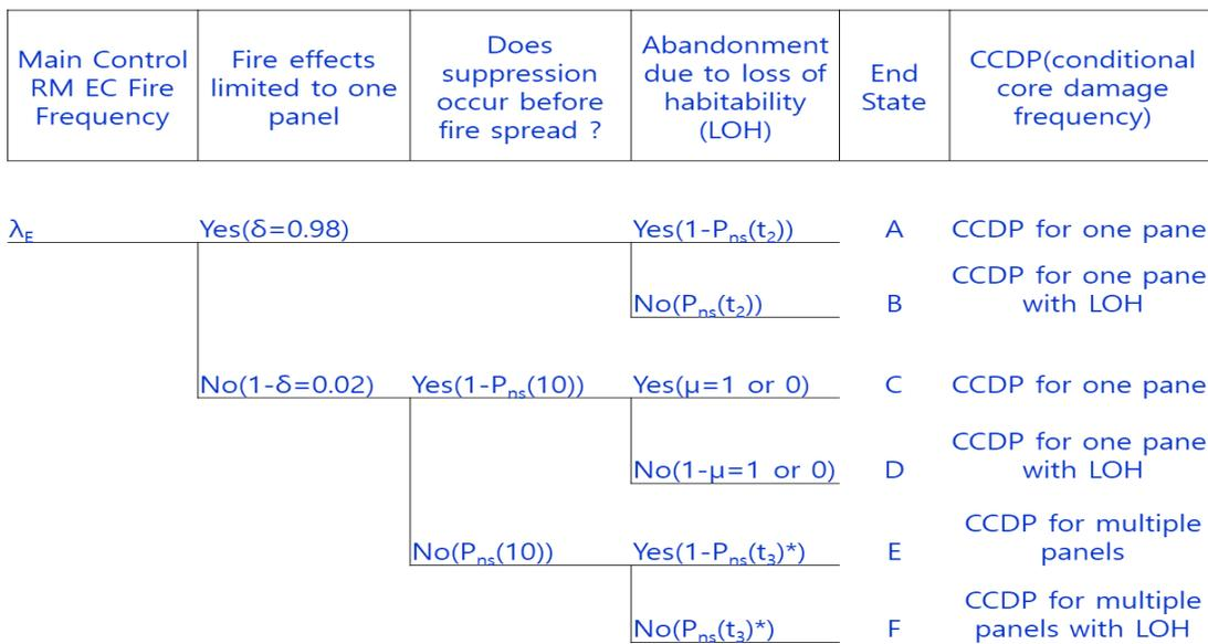
Fig. 3. Event Tree of Electrical Cabinet Fire in MCR
