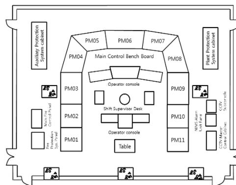
Fig.1. Overview of the MCB for the reference NPP
