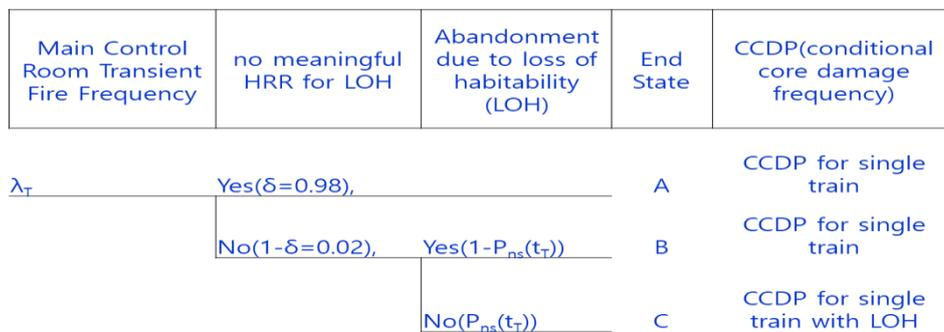
Fig. 4. Event Tree of Transient Fire in MCR
