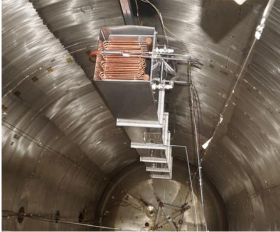
Fig. 5. Installation of a heat-sink in the SPARC vessel
