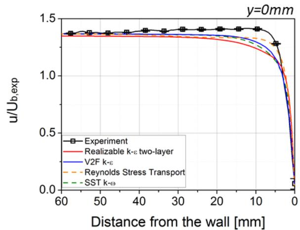
Fig. 6. Vertical velocity profiles at the mid-plane of the test section for the case C.
