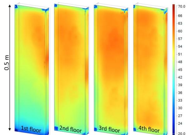
Fig. 1. One of the captured temperature distributions on the outer surface of test section.
