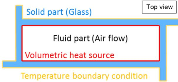
Fig. 2. The concept of boundary conditions in CFD analysis modelled on the test section of the visualization experiment.
