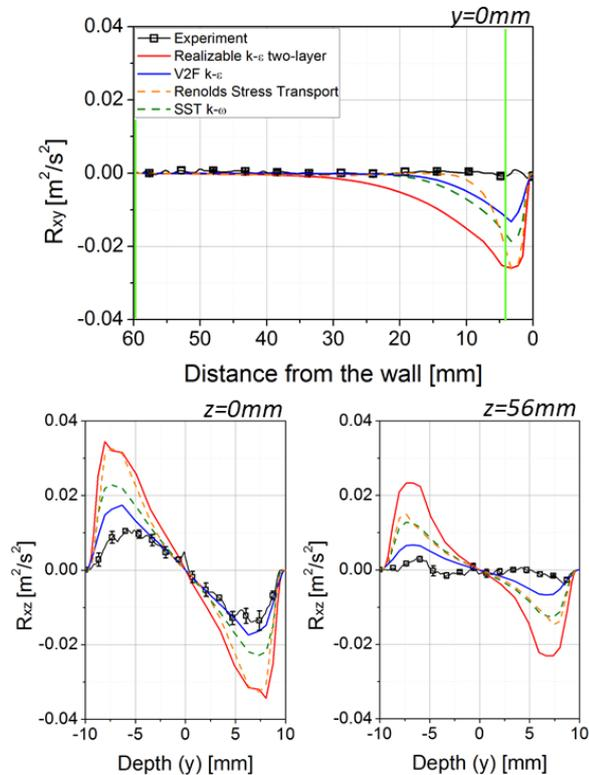
Fig. 7. Reynolds shear stress profiles at  $y = 0$  mm,  $z = 0$  mm and  $z = 56$  mm for the case C.
