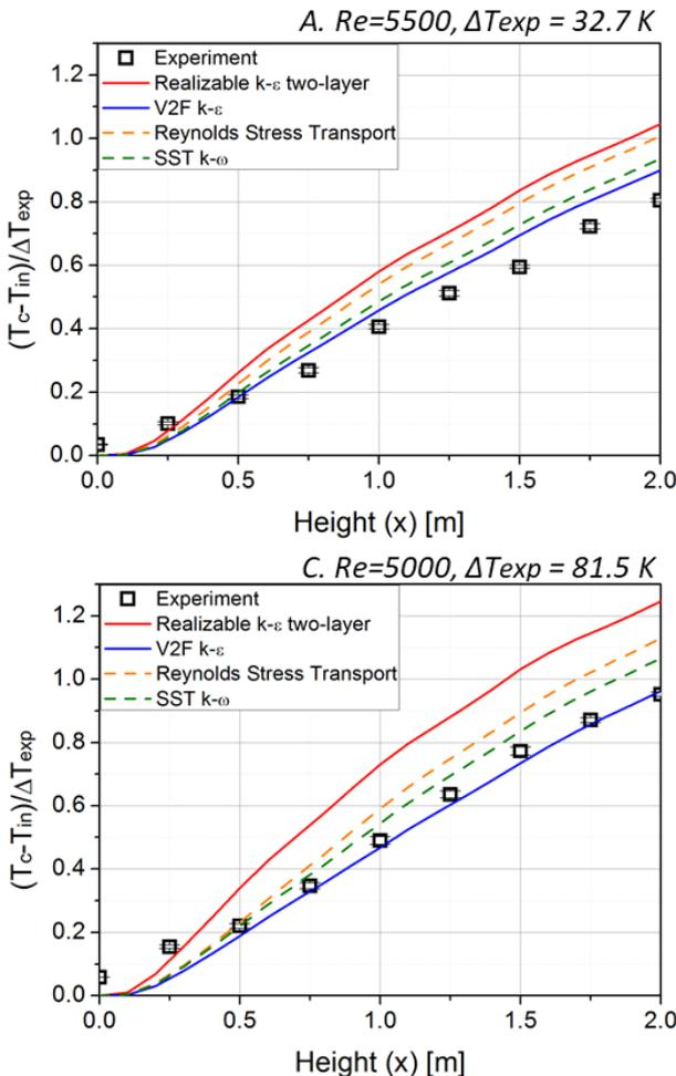
Fig. 5. Local temperature at the center of the test section along the elevation for the case A (up) and C (down).
