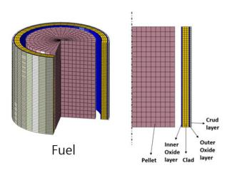
Fig. 3. Concept of oxide/CRUD thermal barrier of high burnup fuel
