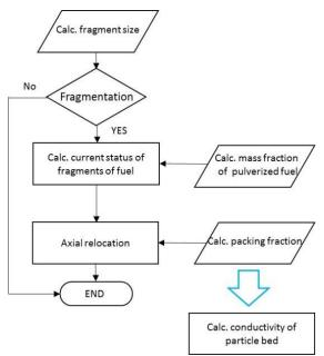
Fig. 2. Calculation flow of QT model
