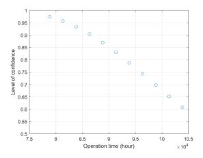
Fig. 1. The level of confidence as a function of operation time  $t_{\gamma}$  with  $\beta = 5$  if reliability goal  $\gamma = 0.95$  is chosen
