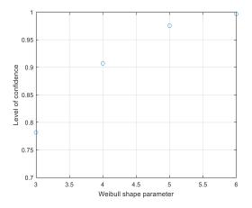
Fig. 2. The level of confidence as a function of  $\boldsymbol{\beta}$  when reliability is 95% and operation time is 78440 hours
