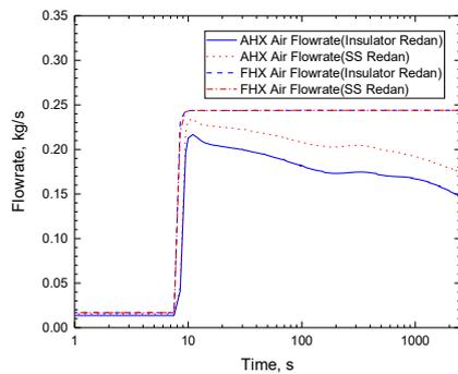
Fig. 10. Change of air flow in DHRS in case of LOF through redan effect
