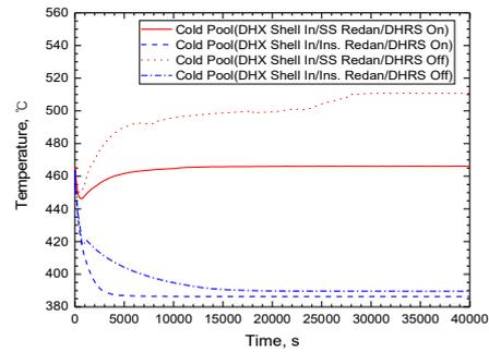
Fig. 8. Cold pool DHX shell temperature Stainless steel redan and Insulator redan in case of DHRS On or Off
