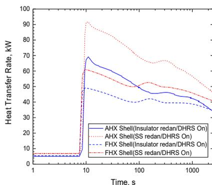
Fig. 11. Heat removal amount of AHX/FHX in case LOF through DHRS on
