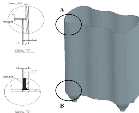
Fig. 2. Detailed Drawing of Redan Structure
