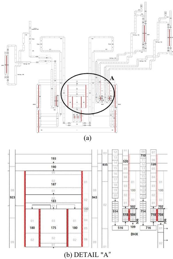
Fig. 3. Nodalization of MARS-LMR code for basic design of STELLA-2.
