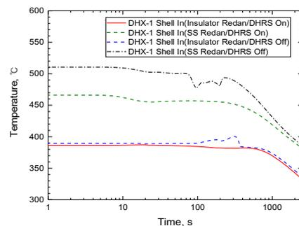
Fig. 9. DHRS DHX shell in cold pool temperature in case of LOF through DHRS on or off
