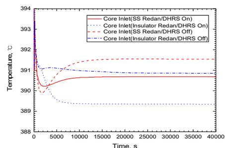
Fig. 5. Core Inlet Temperature
