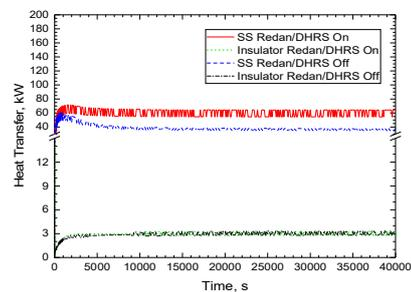
Fig. 4. Heat transfer from hot pool to cold pool through Redan in case of DHRS on or off
