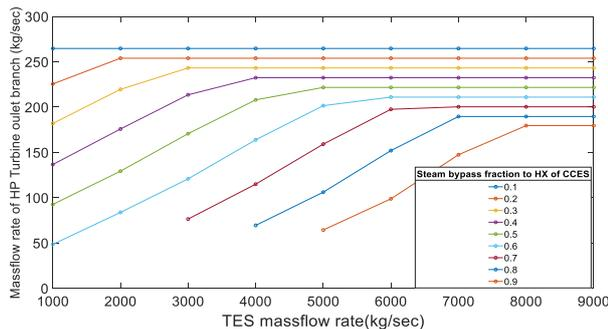
Figure 10. Mass flow rate of HPT outlet branch vs TES mass flow rate (Total steam bypass fraction to CCES: 20%)
