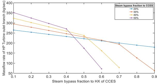
Figure 9. Mass flow rate of HPT outlet branch vs Steam bypass fraction to HX of CCES (TES mass flow rate: 9000kg/sec)
