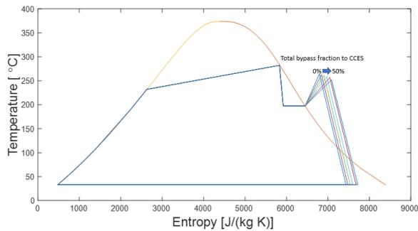
Figure 4. T-s diagram of steam cycle with CCES (Total bypass fraction: 0~50%)
