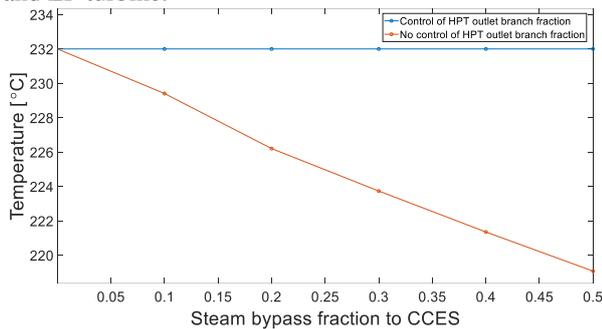
Figure 3. SG inlet temperature vs Total steam bypass fraction to CCES
