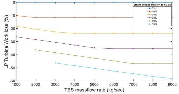
Figure 5. LPT work loss vs TES mass flow rate (Steam bypass fraction to HX of CCES: 0.4)
