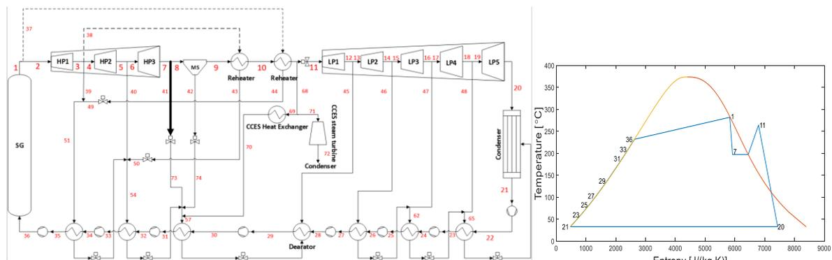
Figure 1. Layout and T-s diagram of Steam Cycle integrated with CCES
