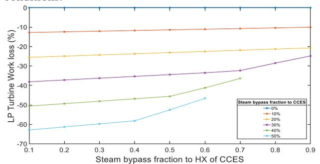
Figure 7. LPT work loss vs Steam bypass fraction to HX of CCES (TES mass flow rate: 9000kg/sec)
