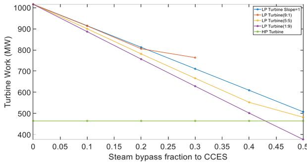
Figure 8. Turbine work vs Total steam bypass fraction (TES mass flow rate: 9000kg/sec)
