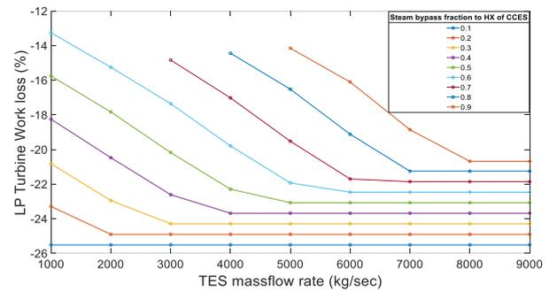
Figure 6. LPT work loss vs TES mass flow rate (Total steam bypass fraction to CCES: 20%)
