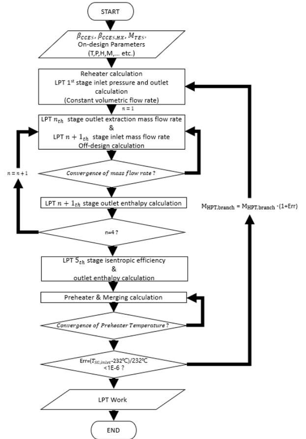
Figure 2. The overall steam cycle flow chart
