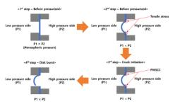
Fig. 3. Brief concept of PWSCC initiation and disk burst in RDT test
