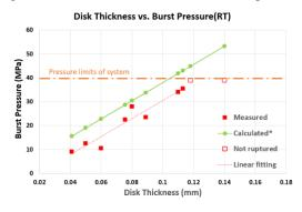
Fig. 6. Burst pressure vs. disk thickness calculated and measured at room temperature.
