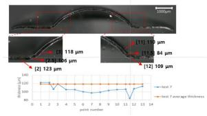
Fig. 9. The thickness change measurement (test 7 - not ruptured specimen)
