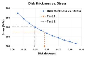
Fig. 10. The applied stress vs. specimen thickness expected from the FEA results
