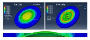
Fig. 8. FEA results of the rupture disk ( $\Phi$  : 10 mm, D : 5mm, t : 0.2 mm)
