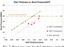
Fig. 7. Burst pressure for disk thickness in high temperature condition.
