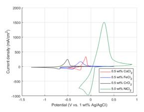
Figure 1. cyclic voltammograms of LiCl-KCl-NiCl<sub>2</sub>, CrCl<sub>2</sub>, FeCl<sub>2</sub>, CoCl<sub>2</sub>. Temperature: 500 °C, v: 300 mV/s
