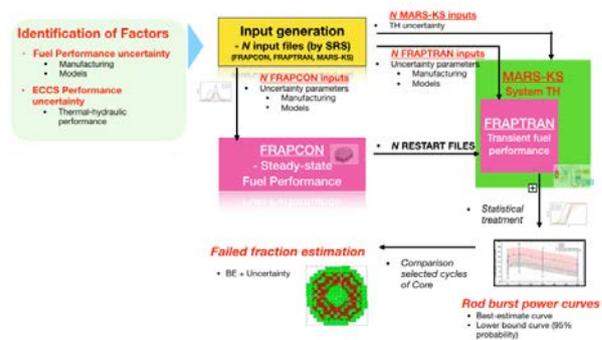
Fig. 1. Schematic drawing of core-wide fuel rod burst analysis methodology [4]
