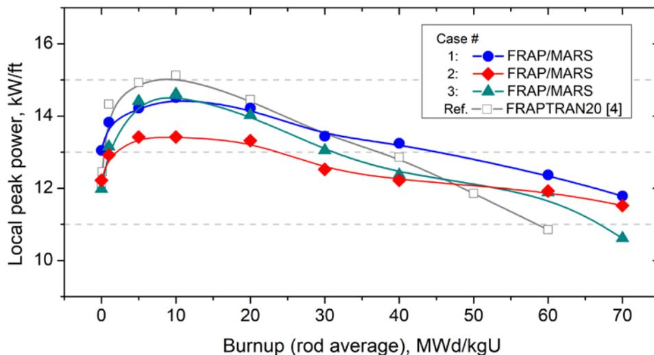
Fig. 1. Best-estimate required peak fuel power for rod burst as a function of fuel burnup with given hot assembly LHGR conditions
