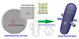
Fig. 1. Mesh generation of RPV using RVMesh-3D
