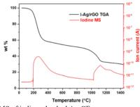
Fig 5. TGA-MS of iodine adsorbed Ag-GF
