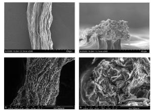
Fig. 1. Axis and cross-section SEM images of graphene fibers(up) and Ag-graphene fibers(down)
