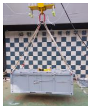
Fig. 2. Drop test of the IP-2 metal rectangular container
