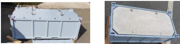
Fig. 1. IP-2 metal rectangular container and simulant of the concrete waste foam
