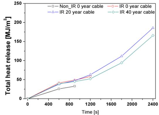
Fig. 2. THR values with respect to time for specimens
