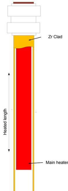
Fig. 3. Assembled heater and cladding
