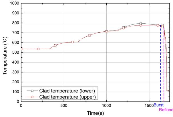
Fig. 10. Clad temperature during burst test
