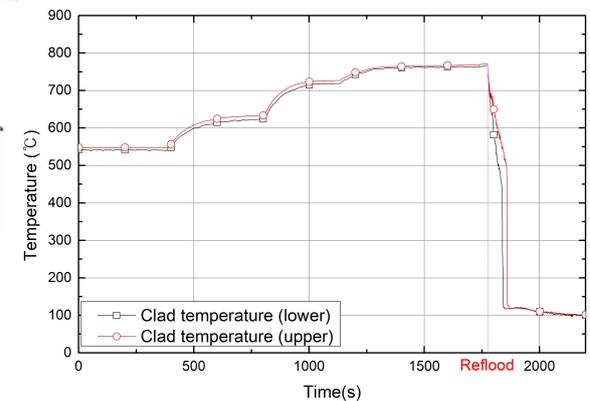
Fig. 6. Clad temperature during reflood test
