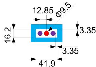
Fig. 2. Cross section of test section (unit: mm)
