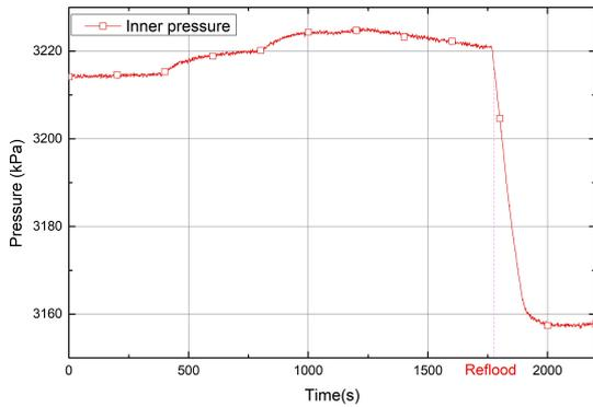
Fig. 7. Inner pressure during reflow test
