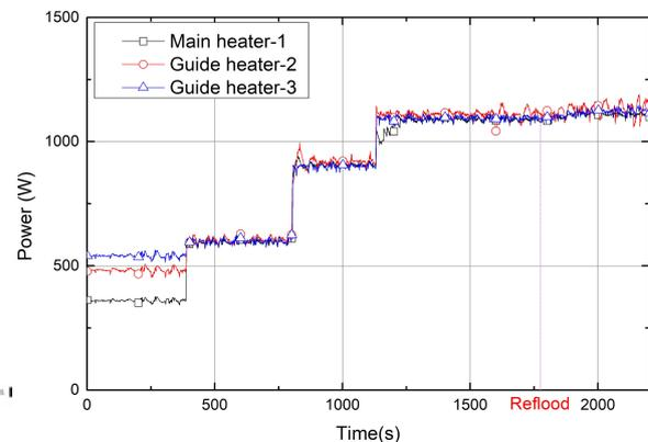
Fig. 5. Applied electric power during reflood test
