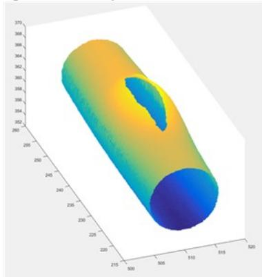
Fig. 12. 3D scan result of burst clad
