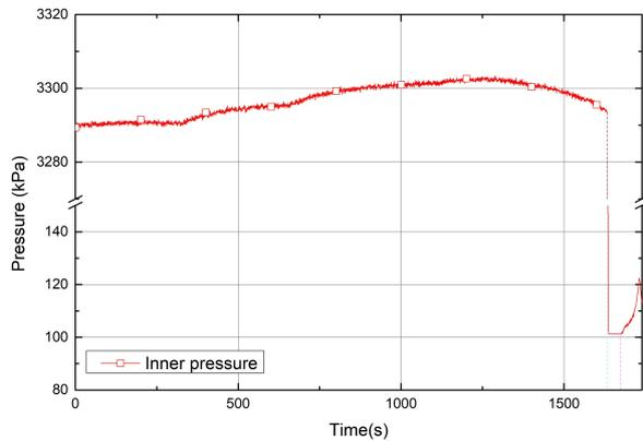
Fig. 11. Inner pressure during burst test
