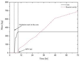
Fig. 4. Hydrogen mass generated in the core and reactor cavity (MLO-SBO)
