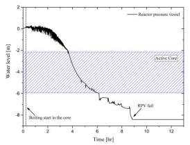
Fig. 2. The water level of the reactor pressure vessel (MLO-SBO)
