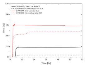
Fig. 6. Cs mass chemisorbed in the RCS (MLO-SBO, FPO-SBO)
