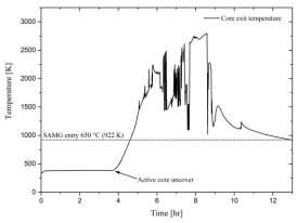
Fig. 3. Maximum core exit temperature (MLO-SBO)
