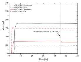
Fig. 5. Total Cs mass in the containment and RCS (MLO-SBO, FPO-SBO)
