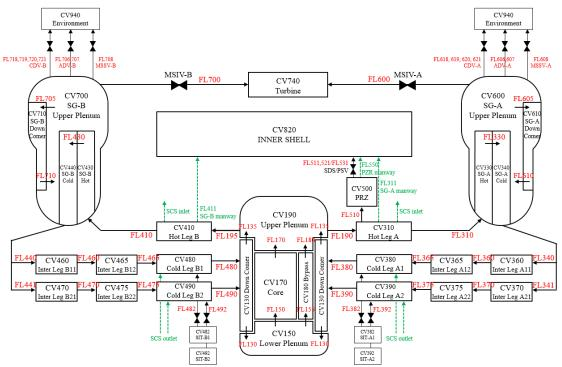
Fig. 1. The RCS nordalization of OPR1000 MELCOR model
