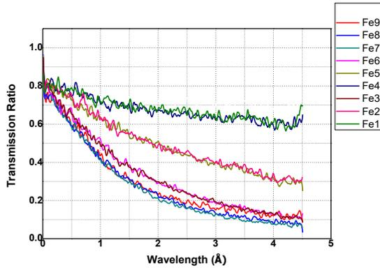
Fig. 3. Neutron transmission ratio of prepared samples in accordance with neutron wavelength
