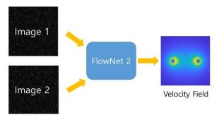
Fig. 4. The process of PIV estimation using FlwoNet2
