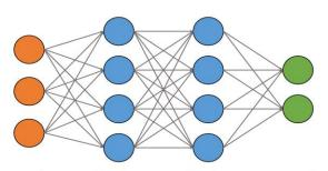
Input layer Hidden layer 1 Hidden layer 2 Output layer Fig. 1. A simple sketch of the deep neural network
