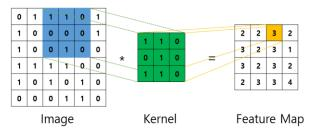
Fig. 3. The process of convolution operation.
