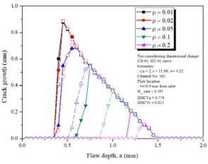
Fig. 7. Crack growth evaluation by DHC.
