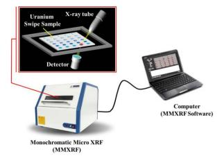
Fig. 1. MMXRF (Monochromatic Micro-focusing XRF)
