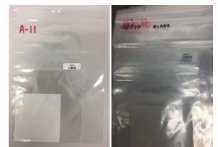
Fig. 2. Examples of IAEA blind test swipes
