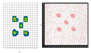
Fig. 5. 2D map uranium contents in a point swipe measured by IAEA TRIPOD (left) and MMXRF (right)
