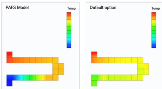
Fig. 6. Distribution of fluid temperature inside PCHX at 300 sec after PAFS operation
