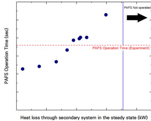
Fig. 3. Comparison of PAFS operation time according to heat loss through the secondary system
