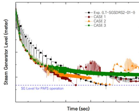
Fig. 4. Comparison of Steam Generator Level with 3 Cases
