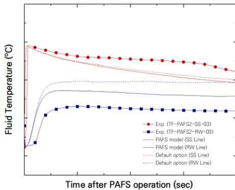
Fig. 5. Fluid temperature at SS line and RW line after PAFS operation
