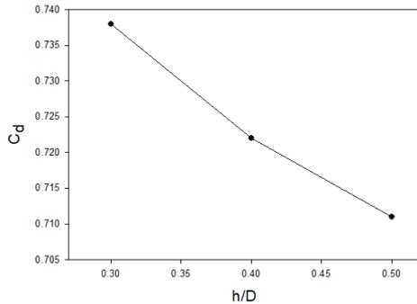
Fig. 6. Discharge coefficient data for wedge flowmeters with different h/D ratios
