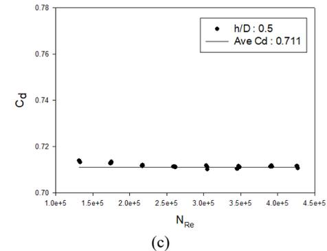
Fig. 5. Discharge coefficient data for flow rate of wedge flowmeters with h/D ratios of 0.3(a), 0.4(b), and 0.5(c)
