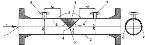
1-Flow, 2-Meter body, 3-Meter body centerline, 4-Wedge element, 5-Wedge apex, 6-High pressure tapping, 7-Low pressure tapping
