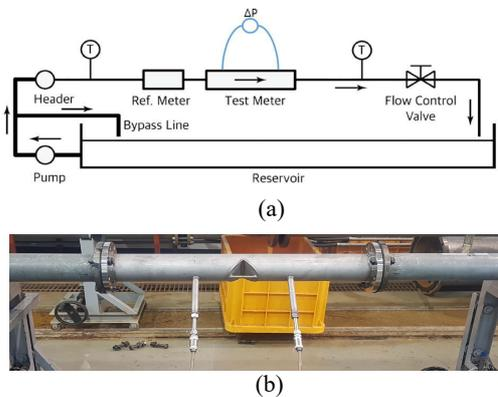
Fig. 3. Schematic diagram (a) and photograph(b) of experimental apparatus
