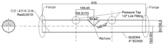
Fig. 2. Schematic diagram of wedge flowmeter
