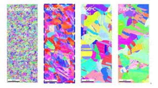
Fig. 1. Texture analysis of heat treated billet (L direction)
