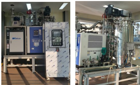
Fig. 2. Drying Facility of Centrifugal Thin-Film Type
