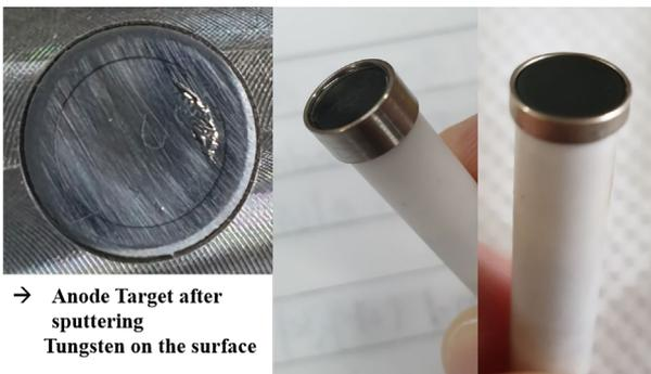
Fig. 6. Left - developed Flat-shaped anode target (Tungsten sputtered) Right – developed flat target miniature X-ray tube
