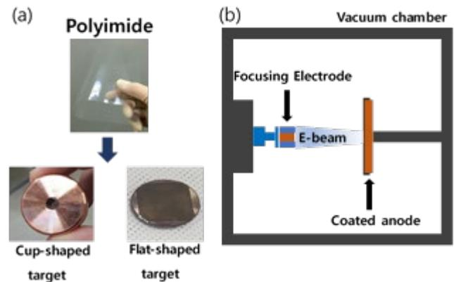
Fig. 2. (a) Cup-type & Flat-type anode target polyimide coating preparation (b) Focal spot size measurement test schematic
