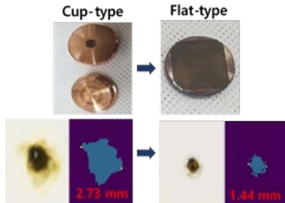
Fig. 3. Focal spot size comparison between cup & flat target
