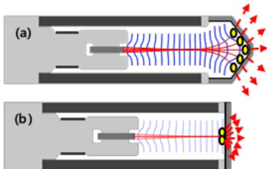
Fig. 1. (a) X-ray tube with cup-type anode target
