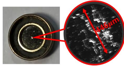
Fig. 7. Real focal spot size from irradiation of developed flat target X-ray tube (Longest: 446  $\mu\text{m}$ , Shortest: 248 $\mu\text{m}$ )
