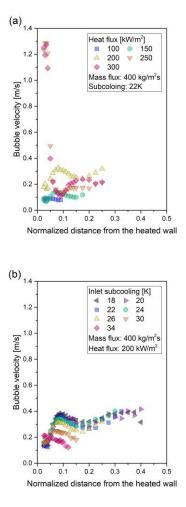
Figure 2. Bubble velocity with varying heat flux (a) and inlet subcooling (b) [1]
