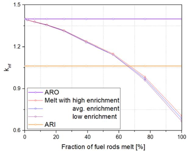
Fig. 3. Sensitivity of the criticality on the various enrichment of the fuel melt (Case 1)
