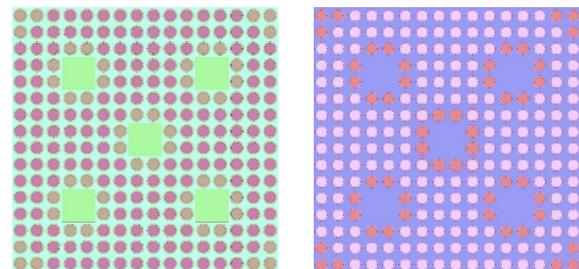
(a) Fuels in the part of the control rods relocated
