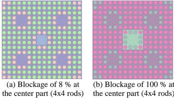
Fig. 2. Modeling for the sensitivity analyses on the amount of blockage
