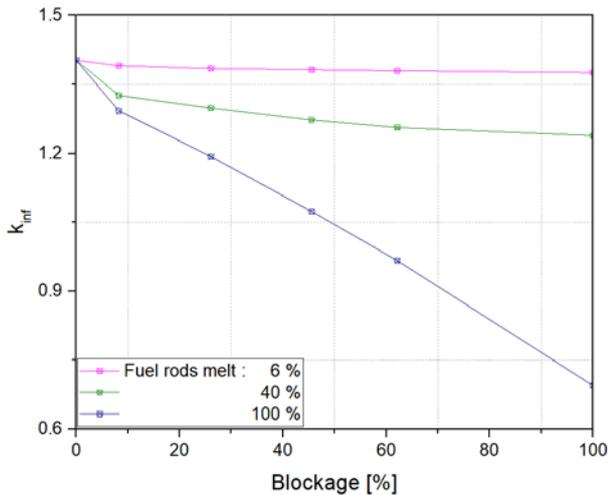
Fig. 6. Sensitivity on the amount of the blockage (Case 4)
