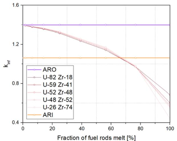
Fig. 4. Sensitivity of the criticality on the various fractions of U and Zr (Case 2)
