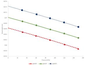
Fig. 4. Wavelength of FBG for system pressure measurement including temperature induced wavelength shift at each temperature
