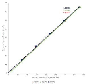
Fig. 6. The percentage of full scale accuracy of the developed pressure transmitter with temperature compensation versus the reference pressure transmitter
