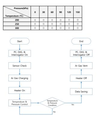
Fig. 3. Test procedure
