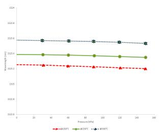
Fig. 5. Wavelength of FBG for temperature compensation at each temperature without pressure induced wavelength shift
