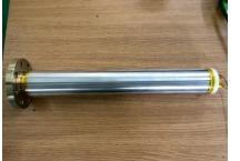
Fig. 1. The prototype of FBG-based pressure transmitter
