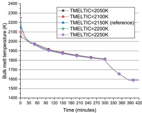
Fig. 9. Bulk Melt Temperature according to Initial Melt Temperature (TMELTIC)
