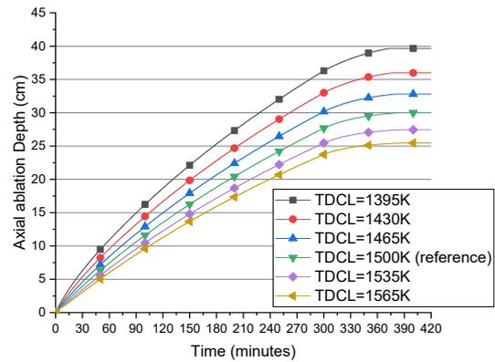
Fig. 6. Axial Ablation Depth according to Concrete Decomposition Temperature (TDCL)
