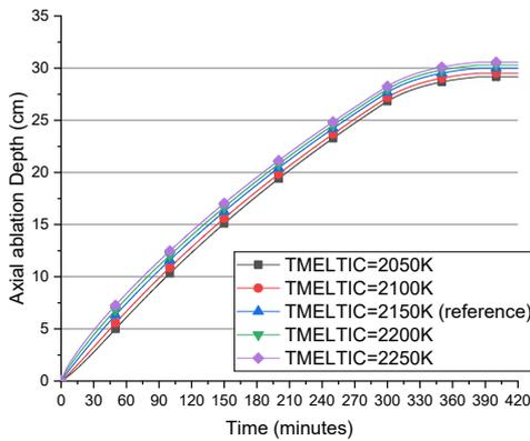
Fig. 8. Axial Ablation Depth according to Initial Melt Temperature (TMELTIC)
