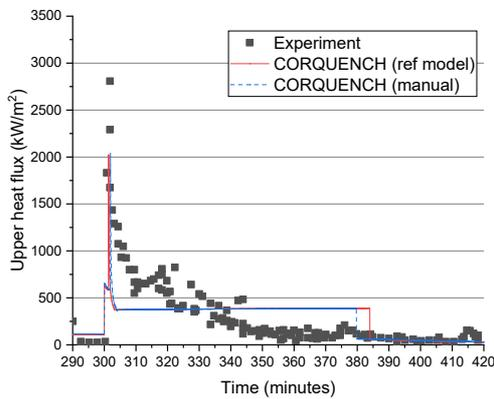
Fig. 3. Comparison of Upper Heat Flux
