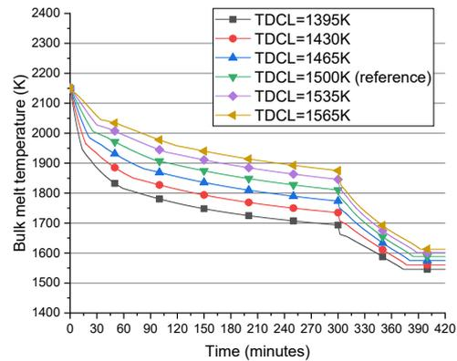
Fig. 7. Bulk Melt Temperature according to Concrete Decomposition Temperature (TDCL)
