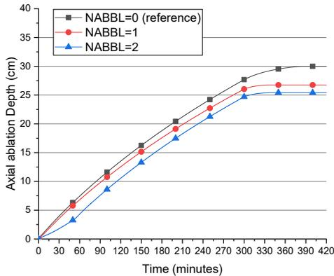
Fig. 4. Axial Ablation Depth according to Concrete Ablation Model (NABBL)
