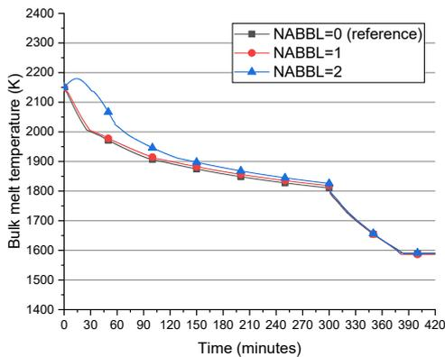
Fig. 5. Bulk Melt Temperature according to Concrete Ablation Model (NABBL)
