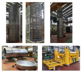
Fig. 1. Test model fabrication (a) canister (b) internal structure (c) installation of disks into canister (d) cask (e) cradle.
