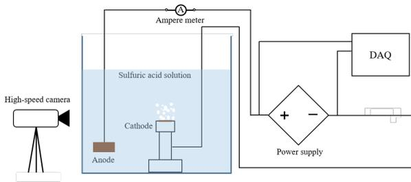
Fig. 1. Experimental apparatus and test section.
