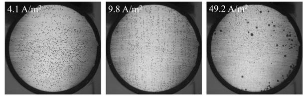
Fig. 2. Hydrogen bubble behaviors on the cylindrical ribbon.
