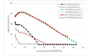
Fig. 3. AFS fuel mechanical and thermal gap between pellet and cladding vs. local burnup
