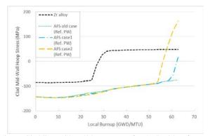
Fig. 7. Cladding mid-wall hoop stress for AFS with reference rod power history
