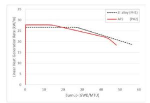
Fig. 1. Bounding power histories for Zr-based alloy cladding and AFS cladding fuel rods.
