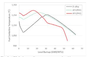
Fig. 2. AFS fuel centerline temperature vs. local burnup
