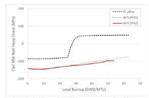
Fig. 4. AFS cladding mid-wall hoop stress vs. local burnup
