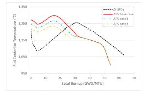
Fig. 5. Fuel centerline temperature calculation result for AFS gap size optimization
