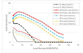
Fig. 6. Mechanical and thermal gap between pellet and cladding calculation result for AFS gap size optimization
