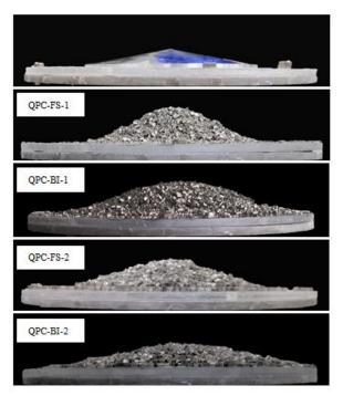
Fig. 4: Snapshot of debris bed for different QPC tests cases
