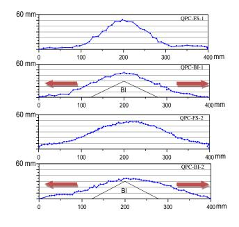
Fig. 5: Measured height of debris bed for test different cases
