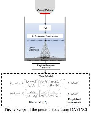
tests with bottom inclination
