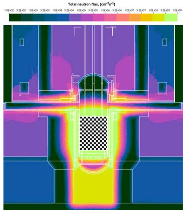
Fig. 4. Total neutron flux distribution for the NPP Beznau [4] (legend ends at 1.0E+09)
