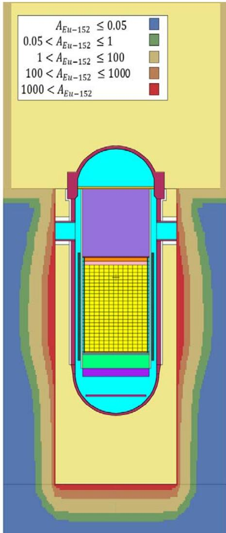
Fig. 2. Eu-152 activity distribution [Bq/g] for concrete structures of Kori-1(A) (13 y decay)
