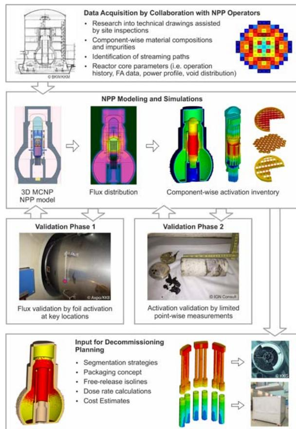
Fig. 1. Scheme of the Advanced Methodology for Activation Characterization (AMAC)
