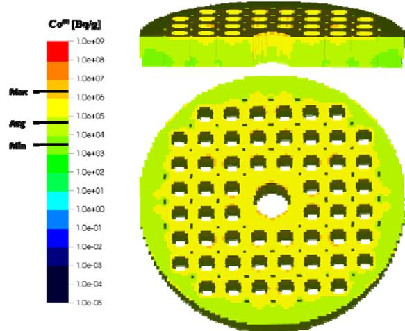
Fig. 3. Illustrative specific Co-60 activity distribution in the lower core support plate, based on Kori-1(A) activation calculation and Beznau detailed geometry and AMAC results (10 y decay)
