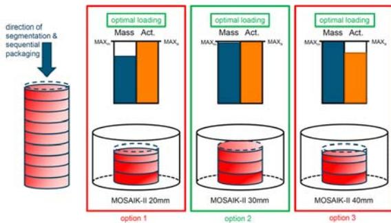
Fig. 7. Evaluation of different waste container loading options by the NAGRA optimization code ALGOPACK
