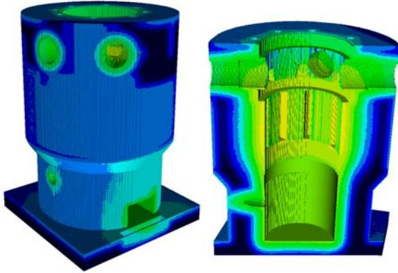
Fig. 5. Realistic activation distribution pattern for the wall and floor of the NPP Beznau biological shield [1]
