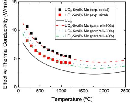
Fig. 3. Comparison of thermal conductivity data with calculated curves using equation (1)
