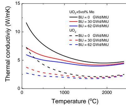
Fig. 5. Estimation of burnup effect on effective thermal conductivity
