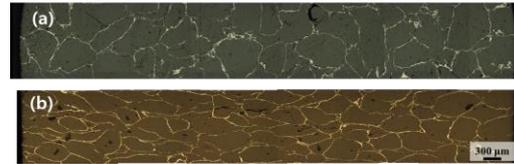
Fig. 2. Pellet microstructures vertical to (a) axial direction and (b) radial direction
