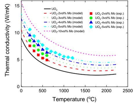
Fig. 4. Comparison of thermal conductivity data with calculated curves obtained using equation (3)
