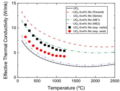
Fig. 1. Thermal conductivity of UO<sub>2</sub>-5vol% Mo sample and comparison with basic analytical model values
