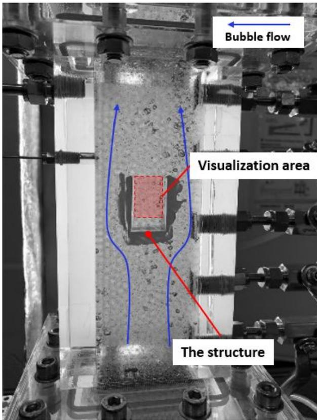
Fig. 4. Test section image with the structure for visualization
