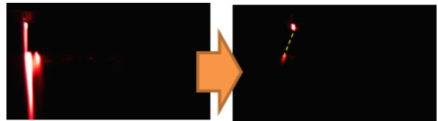
Fig. 2. High speed images with a bended plasma arc
