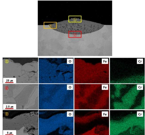
Fig. 4. EDS mapping results on the cross-sectional images of nodular oxidation area of Fe20Cr in 8 hr test
