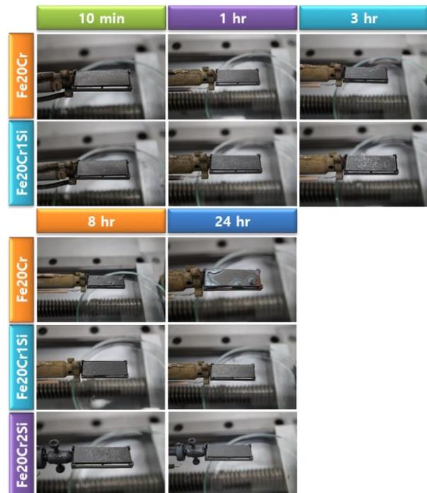
Fig. 1. Surface morphology of FeCrSi alloys after oxidation test and cooling for 1 hr
