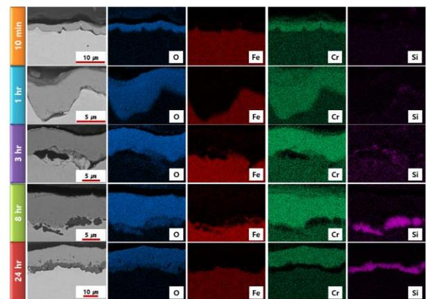
Fig. 5. EDS mapping results on the cross-sectional images of oxide layers of Fe20Cr1Si alloy over time
