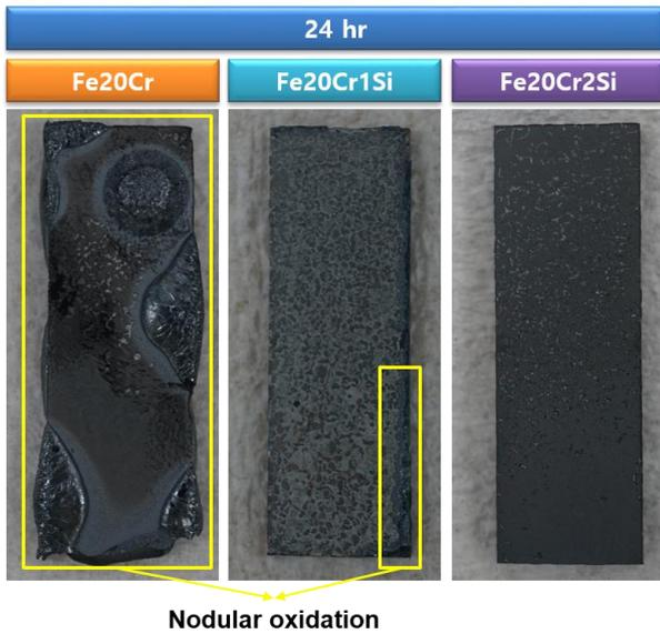
Fig. 2. Comparison of surface morphology of FeCrSi alloys with increasing the Si content after 24 hr test
