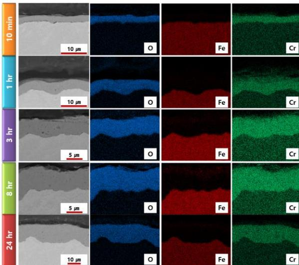
Fig. 3. EDS mapping results on the cross-sectional images of oxide layers of Fe20Cr alloy over time
