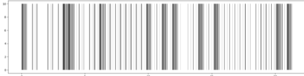
Fig. 3. A printout of all input nuclide number densities in all Fuel Assemblies of a studied LP converted into Barcode format (the values are normalized in range (0,1) and used for grayscale color assignment).
