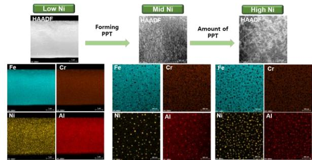
Fig. 1. Precipitations forming behavior according to nickel addition
