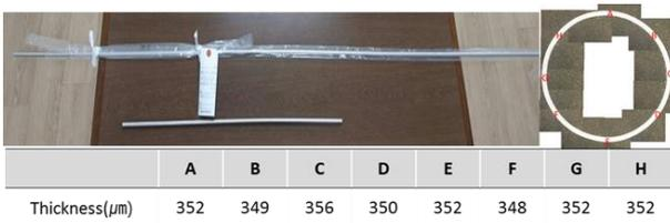
Fig. 4. Photographs of FeCrAl tube fabricated by pilgering with a dimension of 9.5 mm OD x 0.35 mm t x 1.9 m L
