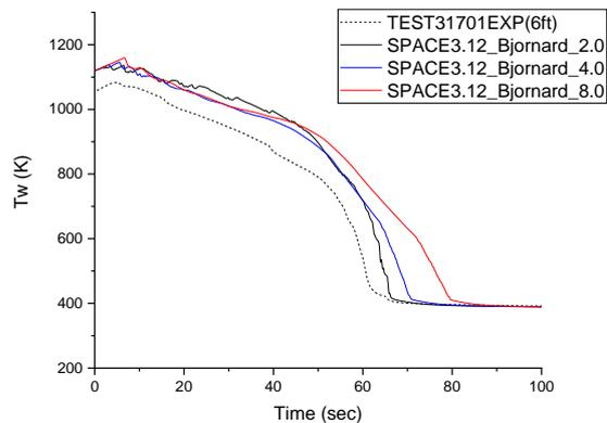
Fig. 6. FLECHT-SEASET Test 31701 results with the various transition boiling heat transfer correlation
