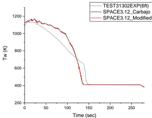
Fig. 7. FLECHT-SEASET Test 31302 results with the modified Carbajo model
