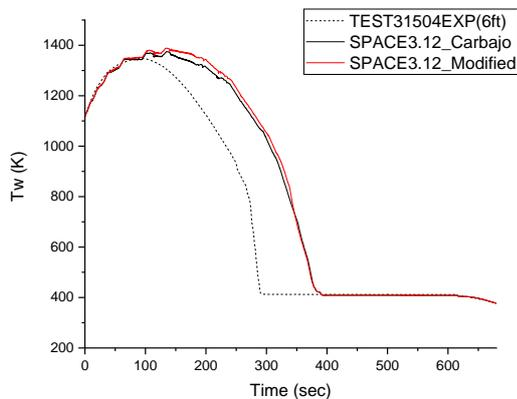
Fig. 8. FLECHT-SEASET Test 31504 results with the modified Carbajo model
