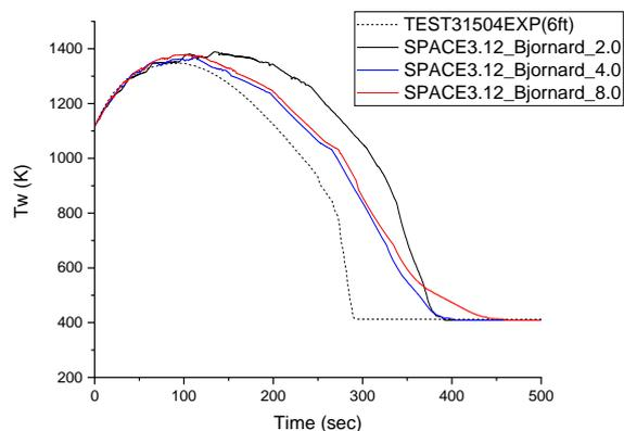
Fig. 5. FLECHT-SEASET Test 31504 results with the various transition boiling heat transfer correlation
