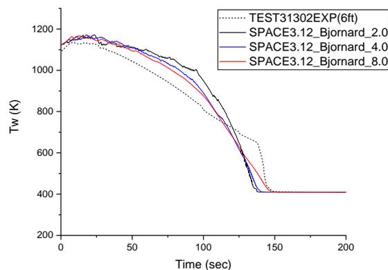
Fig. 4. FLECHT-SEASET Test 31302 results with the various transition boiling heat transfer correlation
