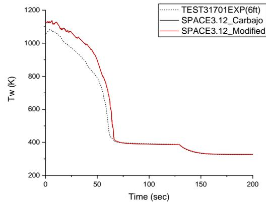
Fig. 7. FLECHT-SEASET Test 31701 results with the modified Carbajo model
