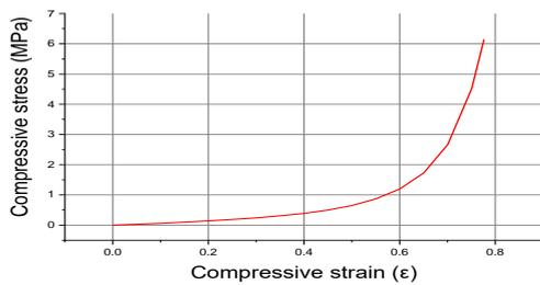
Fig. 3. stress-strain curve of rubber
