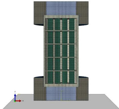
Fig. 2. FE model of transport cask
