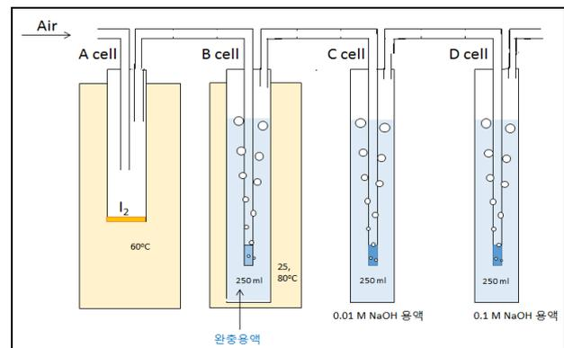
Fig. 3 Scrubbing test facility
