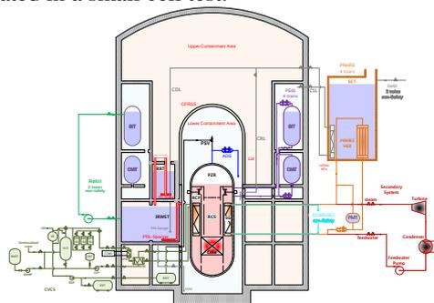
Fig.1 Containment pressure and radioactivity suppression system of SMR
