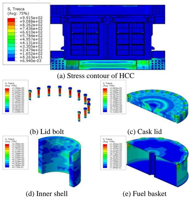
Fig. 3 Stress Contour of 0.3m Base Drop
