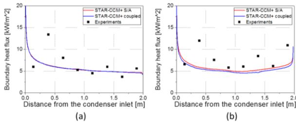
Fig. 6. Comparison between calculated and experimental heat fluxes: natural convective condensation
