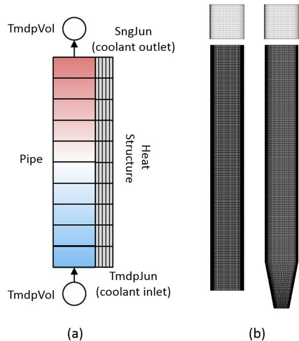
Fig. 4. Sketch of node and meshes of MARS-KS/STAR-CCM+ coupled code analysis
