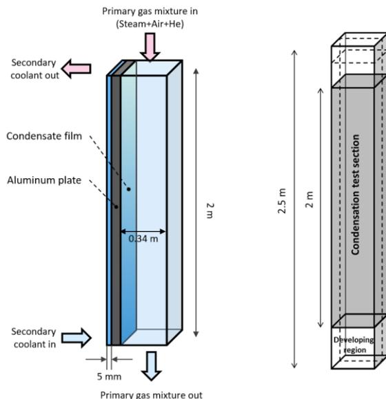
Fig. 3. Sketch of the CONAN facility test section and computational domain of CFD analysis
