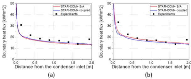
Fig. 5. Comparison between calculated and experimental heat fluxes: forced convective condensation
