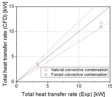
Fig. 7. Comparison of total heat transfer rate between calculated and experimental results
