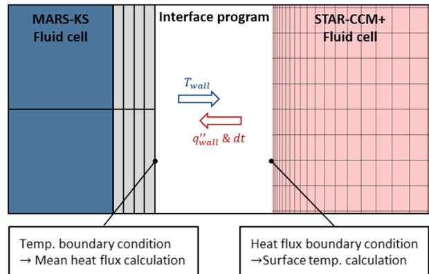
Fig. 2. Diagram of the heat structure coupling method
