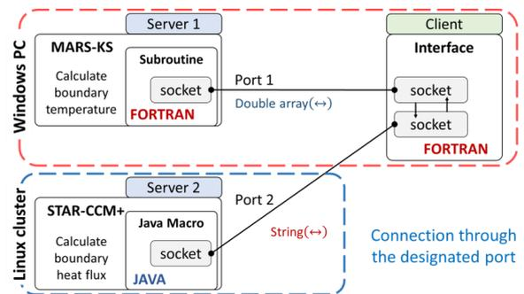
Fig. 1. System & CFD code coupling with socket communication scheme
